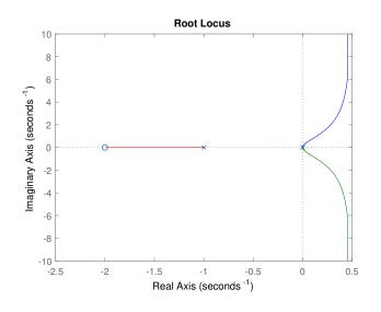
Finally, we consider  $0 \le K_p < K_d$ . Then the departure angles of the two poles at the origin are still  $\pm 90 \text{ deg}$ , and center of the asymptotes lies on the negative real axis, which implies that  $0 \le K_p < K_d$  now stabilizes the closed loop system. For example, the root locus with  $K_p = 0.5K_d$  looks like the following.
