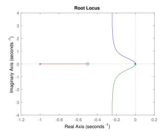
Therefore the only case that stabilizes the closed loop system is  $0 \le K_p < K_d$  with  $K_d > 0$ .
