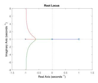
Now we consider  $K_p \geq K_d$ . Then the departure angles of the two poles at the origin are  $\pm 90 \deg$ , and center of the asymptotes lies on the non-negative real axis, which implies that  $K_p \geq K_d$  also fails to stabilize the closed loop system. For example, the root locus with  $K_p = 2K_d$  looks like the following.
