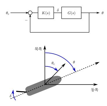
The heading angle dynamics with respect to the fin deflection are described by:
